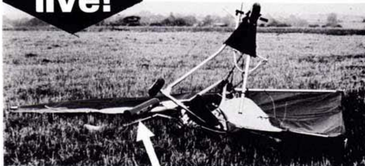
The wreckage of John Clarke's Sabre trike unit — the kingpost was driven 12" into the ground. Note the empty Skymaster container — oh for a double-barrelled model!
