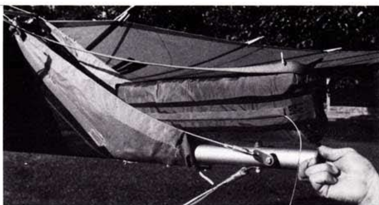
The Dietl parachute in its container in the keel pocket (see Germany)
